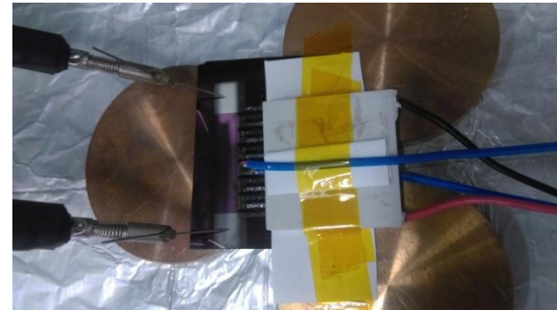
Fig. 3-1. Experimental set-up for determining Seebeck Coeff.
